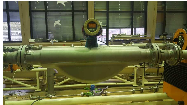
Transfer standard, Coriolis flowmeter, Endress + Hauser / DN 100
