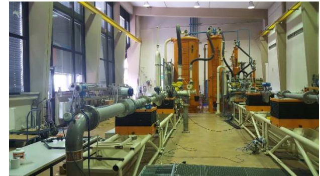
Hydrocarbon flow calibration facility in PTB
